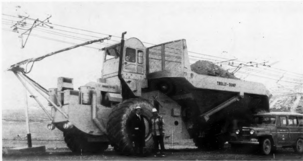
ELECTRIC DUMP truck uses electric power from overhead trolley installation to run 400 hp, direct current LeTourneau
